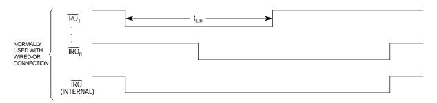
**b. Level-Sensitive Trigger Condition.** If after servicing an interrupt the  $\overline{\text{IRQ}}$  remains low, the next interrupt is recognized.
