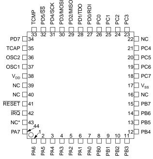
If MC68HC705C8A OTPs are to be used in the same application, this pin should be tied to V<sub>DD</sub>.
