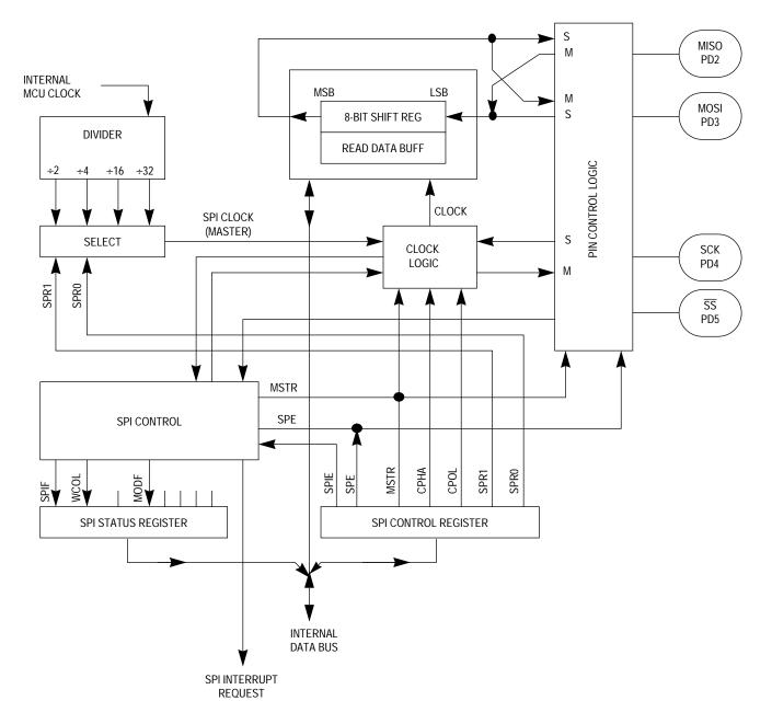
Figure 10-2. Serial Peripheral Interface Block Diagram
