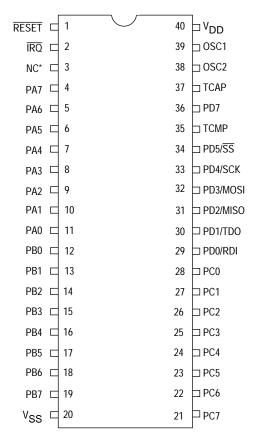
$<sup>^{\</sup>star}$  If MC68HC705C8A OTPs are to be used in the same application, this pin should be tied to  $V_{DD}. \\$
