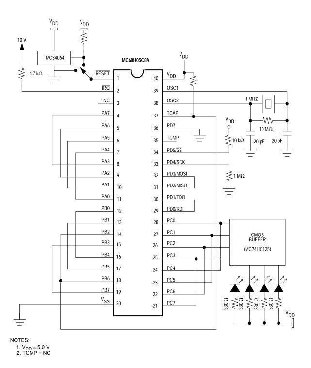
Figure 11-2. Self-Check Circuit Schematic
