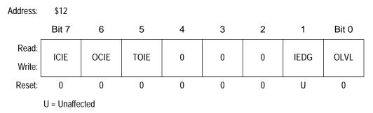
Figure 8-4. Timer Control Register (TCR)
