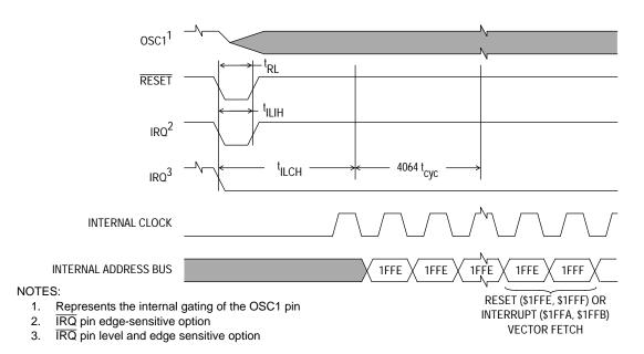
Figure 6-2. Stop Recovery Timing Diagram
