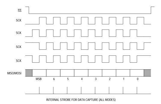
Figure 10-1. Data Clock Timing Diagram
