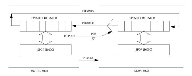
Figure 10-3. Serial Peripheral Interface Master-Slave Interconnection
