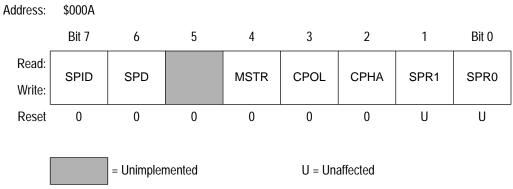
Figure 10-4. SPI Control Register (SPCR)
