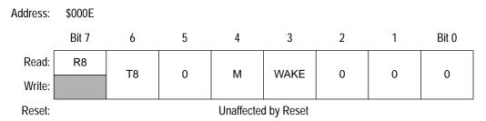
Figure 9-5. SCI Control Register 1 (SCCR1)
