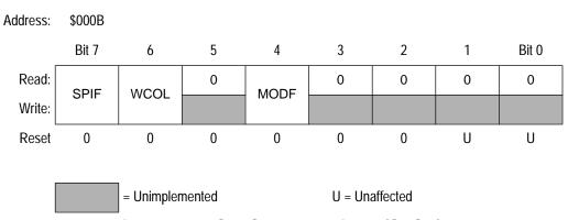
Figure 10-5. SPI Status Register (SPSR)
