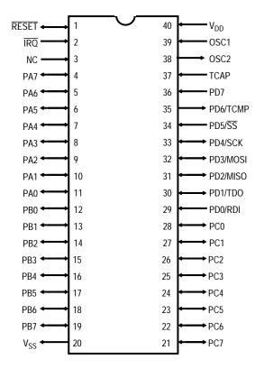
Figure 11-1. User Mode Pinout
