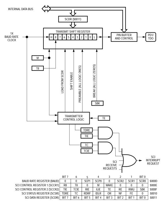
Figure 9-2. SCI Transmitter
