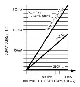
Figure 13-3. Maximum Supply Current Versus Internal Clock Frequency,  $V_{\rm DD}$  = 3.6 V
