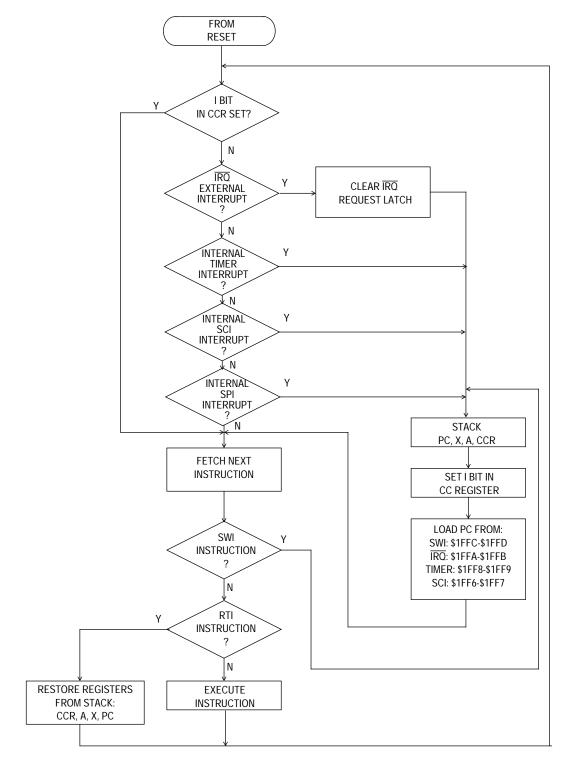
Figure 4-1. Interrupt Flowchart
