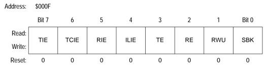
Figure 9-6. SCI Control Register 2 (SCCR2)
