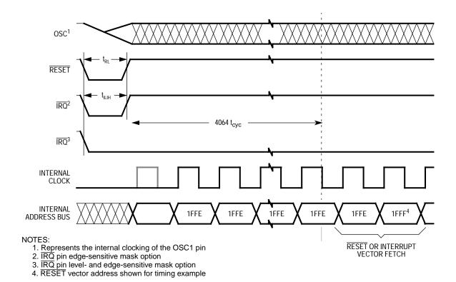
Figure 13-7. STOP Recovery Timing Diagram
