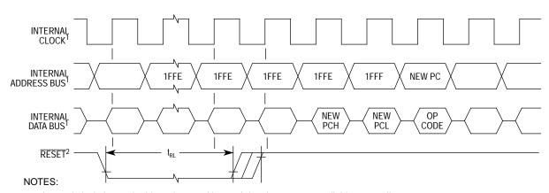
Figure 13-5. External Interrupt Timing
