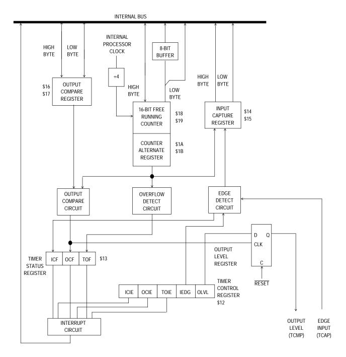
Figure 8-1. Timer Block Diagram
