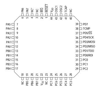
$<sup>^{\</sup>star}\,$  If MC68HC705C8A OTPs are to be used in the same application, this pin should be tied to  $V_{DD}.$
