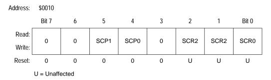
Figure 9-8. Baud Rate Register (BAUD)
