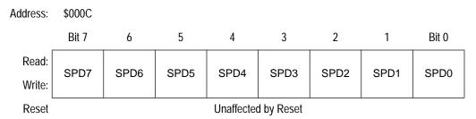
Figure 10-6. SPI Data Register (SPSR)
