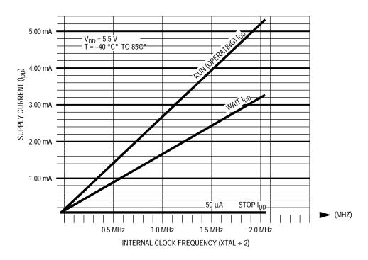
Figure 13-2. Maximum Supply Current Versus Internal Clock Frequency,  $V_{\rm DD}$  = 5.5 V
