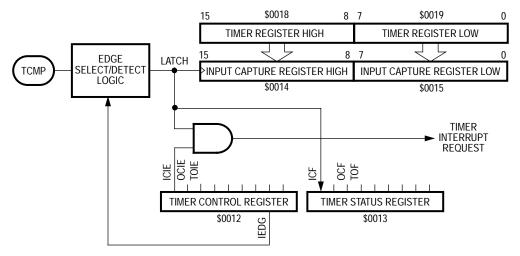
Figure 8-3. Input Capture Operation
